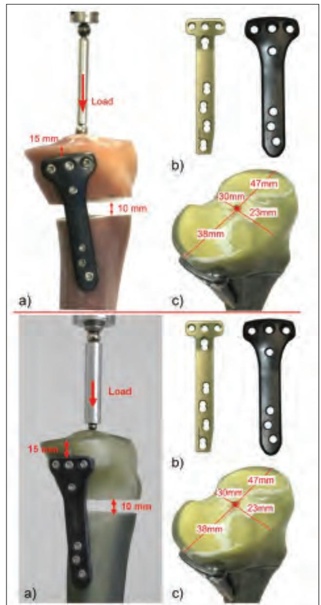
Fig. 1 Experimental set-up with load application and bone gap definition (a, c) for both HTO plates (b)
